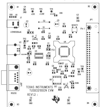
Figure 1-5. TUSB3210 Printed-Circuit Board (REV 1.2)—Top Side
